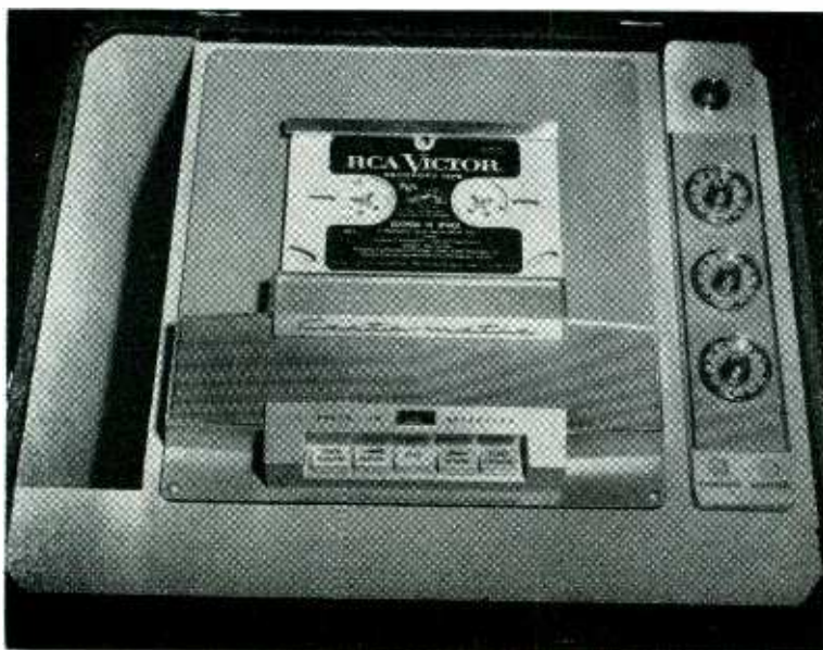
Above, prototype of the RCA cartridge machine which uses the four-track principle and cartridge turnover to play the second set of tracks. Right: four-track Ampex machine with shifting head for playing or recording either two or four tracks. Ampex was first on market with four-track. RCA first with reversible cartridge.
