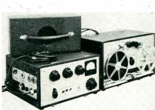
Above is shown two of the "early-birds." At the left is the Ampex 200 which was patterned after the German Magnetophon and right is an early Magnecord, both machines were full track and were used by professionals and radio stations.
